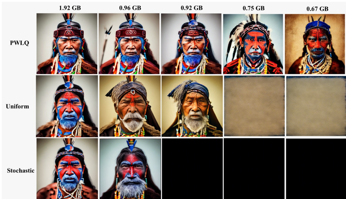
Fig. 6: Comparison of Quantization Methods. Example generated figures are given for piecewise linear (PLWQ), uniform, and stochastic quantization per given model sizes, labeled at the top of columns. The first two model sizes are given by full 16-bit and full 8-bit quantization. The third is 4-bit for convolutional layers and 8-bit elsewhere; the fourth is 4-bit convolutional and transformer layers and 8-bit elsewhere, and the final size is 4-bit convolutional, transformer, and middle U-Net layers, with 8-bit elsewhere. We stop before full 4-bit quantization as that outputs null images for all methods.
